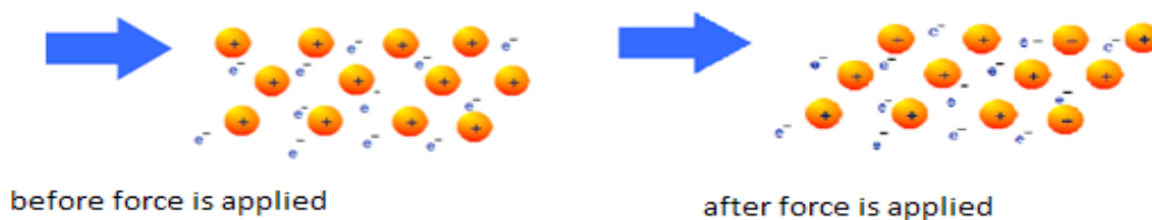
Figure 3.15 Malleability and ductility of metals
