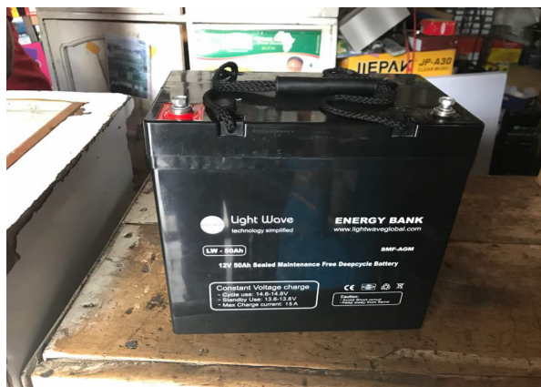
Figure 9.8: Lead acid accumulator battery
